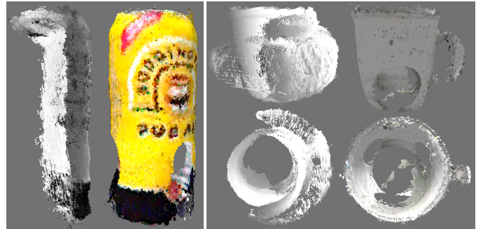
Fig. 7. Shown here are a can and a mug aligned with ICP alone on the left and our algorithm on the right. Due to the high level of symmetry in these objects, ICP is unable to find the correct alignments between depth scans, resulting in useless object models.
