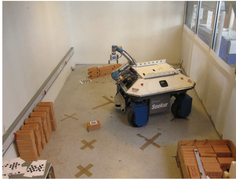
Figure 4.3: The testing environment for developing the masonry application.
