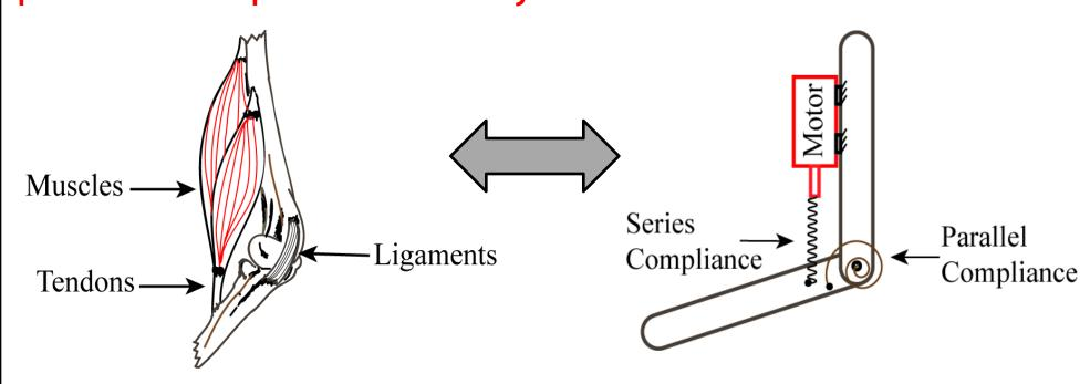
Studies of the metacarpal (MCP) joint show that parallel compliance due to ligaments and joint capsules has a dominant effect on the net passive moment [1].
