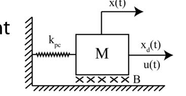
We implemented impedance control at the joint, as it is commonly used for grasping and manipulation tasks,
