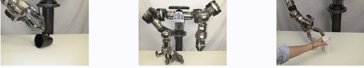
Fig. 1. Potential Manipulations faults. (left) Missed grasp. (middle) Heavy object. (right) Uncontrollable obstacle.
